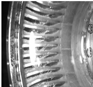
Fig. 12 Camera image of the flow at the inner profile diameter from the turbine to the pump at v=0.8 and s=0.25 .
